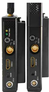
DW-500T Transmitter DW-500R Receiver
